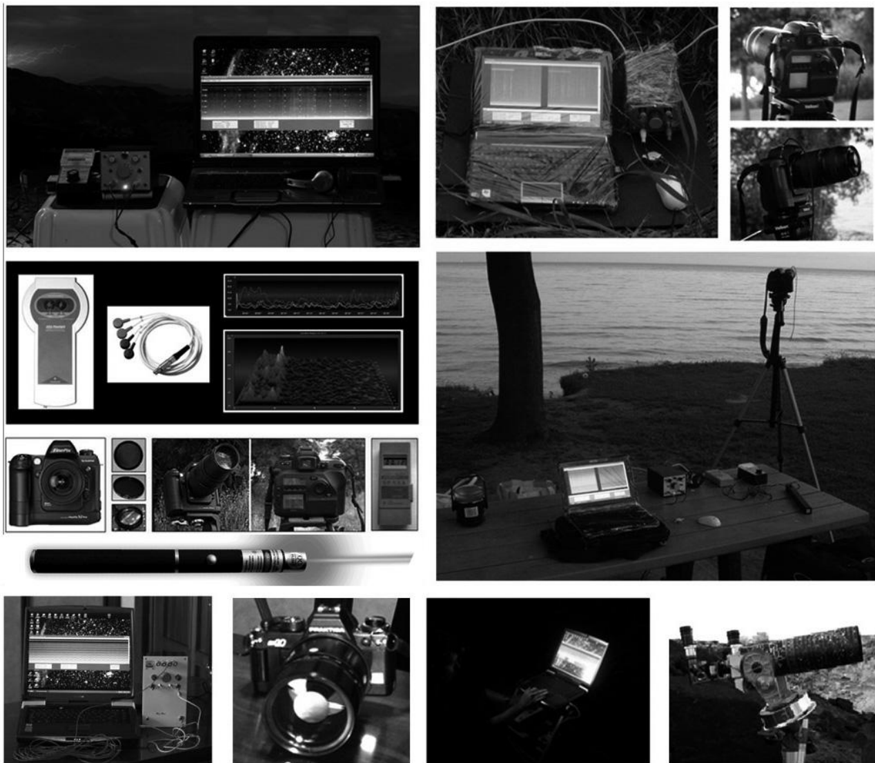
Figure 9. Some of the portable instruments that are currently used more frequently by this author: portable optical photographic and spectrographic equipment, telescopes and catadioptric lenses, polarizing and infrared filters, VLF-ELF spectrometer, analogical magnetometer, Geiger, Laser and EEG.
